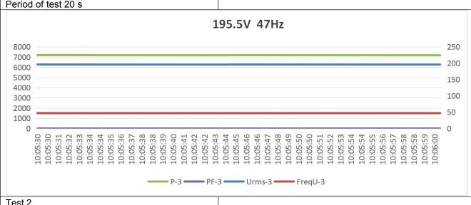
Test 2 Voltage = 85% of nominal (195.5 V), Frequency = 47.5 Hz, Power Factor = 1, Period of test 90 minutes
